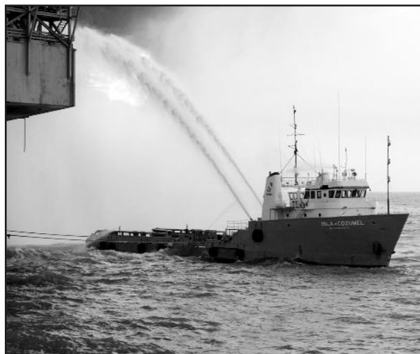
Marine Turbine Technologies' fire suppression pumps sit on this tugboat, circling an oil rig in Cozumel, Mexico, to keep the rig safe from the flame-out of natural gas.
